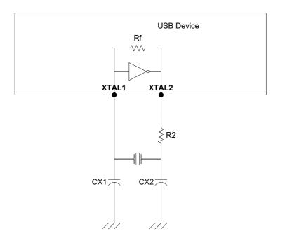
This circuit diagram shows an implementation of Pierce Oscillator on our USB device. The feedback resistor R1 has been integrated into our USB device. This resistor is used to provide DC bias to a CMOS inverter for inversion amplifier operation. Too large an R sets the circuit unstable while too small a resistor makes the amplifier gain small. We have chosen 100 k $\Omega$  for its optimal bias.
